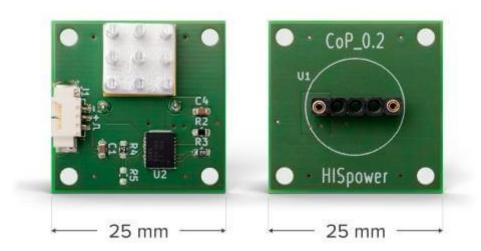
Driver circuit board for a quick evalution of HISpower series IR emitters
