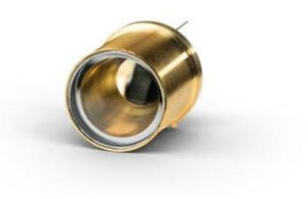
Thermal infrared emitter with Winston cone and soldered BaF<sub>2</sub> window, hermetically sealed
