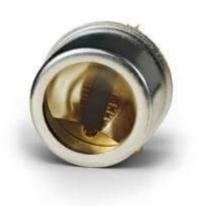
Thermal infrared emitter with CaF2 window, hermetically sealed
