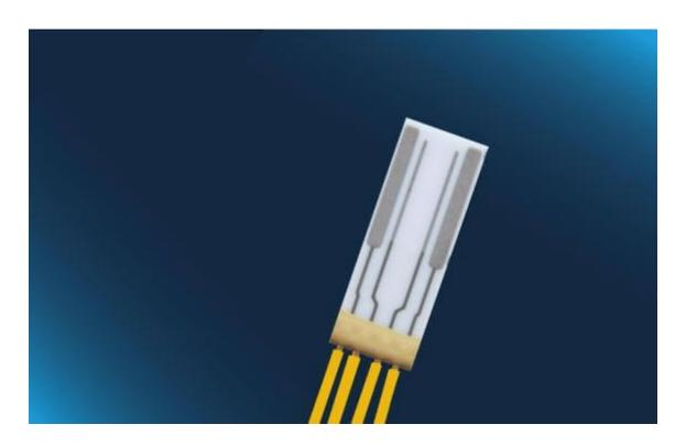
Commodity conductivity sensor with four-electrode measurement for various conductivity measurement applications. Measuring range from 100  $\mu\text{S/cm}$  to 100 mS/cm (typical cell constant of 0.66 cm $^{-1}$ )
