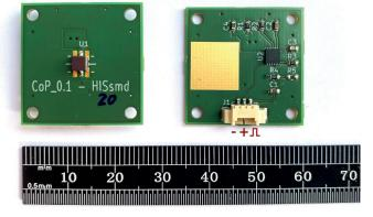
Fig. 2: Driving circuit board for a quick evalution of HISsmd series IR emitters.
