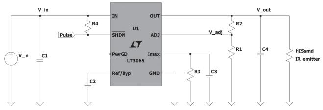
Fig. 1: Application circuit to drive HISsmd series IR emitters with the LDO regulator LT3065
