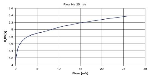
Example - Characteristic for high flow measurement with direction output
