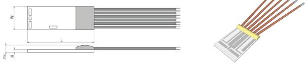
Tolerances: outer dimension (chip):  $\pm$  0.2 mm; thickness (chip):  $\pm$  0.1 mm, height  $\pm$  0.3 mm
