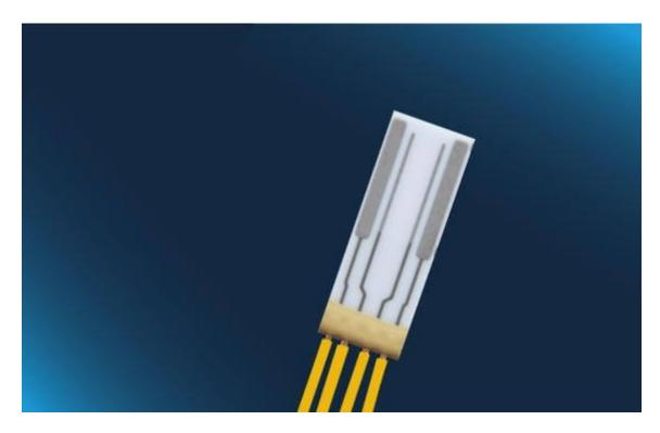
Commodity conductivity sensor with four-electrode measurement for various conductivity measurement applications. Measuring range from 100  $\mu$ S/cm to 100 mS/cm (typical cell constant of 0.66 cm<sup>-1</sup>)
