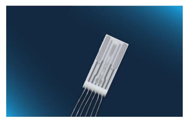
Optimal for applications with a conductivity measuring range from 100  $\mu$ S/cm to 200 mS/cm (typical cell constant of 0.86 cm  $^{-1}$ ) with integrated Pt1000 temperature sensor
