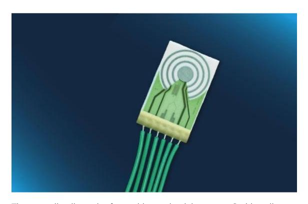
The versatile allrounder for a wide conductivity range: Stable cell constant from low conductivity values ( $10\mu S/cm$ ) to high values 200mS/cm (typical cell constant of 0.42 cm  $^{-1}$ )
