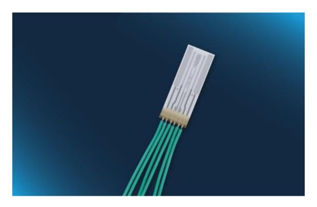
Sensor for Higher Conductivity Ranges with Medium Cell Constant and Integrated Temperature Sensor. Optimal for applications with a conductivity measuring range from  $100~\mu\text{S/cm}$  to 200~mS/cm (typical cell constant of 0.68~cm -1)
