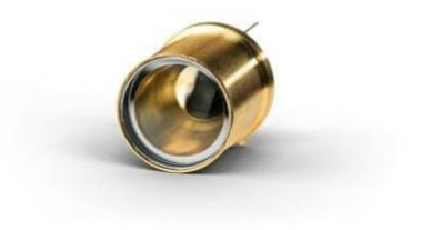
Thermal infrared emitter with Winston cone and soldered CaF<sub>2</sub> window, hermetically sealed
