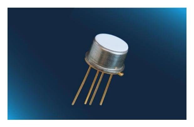
Humidity module with a front PTFE membrane filter for VOC and particle protection.
