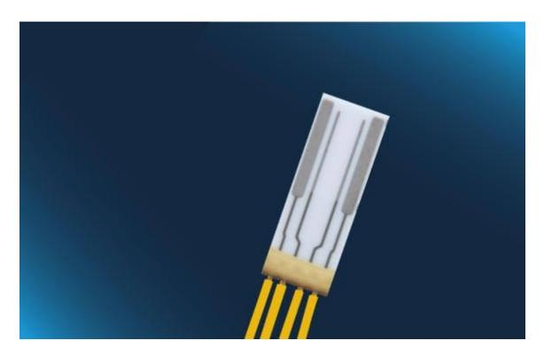
Commodity conductivity sensor with four-electrode measurement for various conductivity measurement applications. Measuring range from 100  $\mu\text{S/cm}$  to 100 mS/cm (typical cell constant of 0.66 cm $^{-1}$ )
