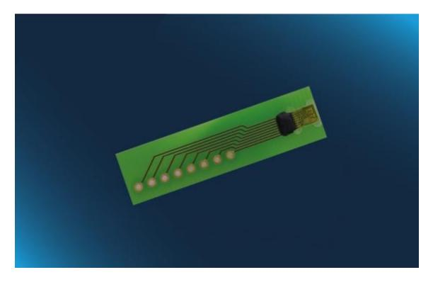
Gas flow sensor with flow range from 0 to 1.5 m/s (full bridge mode), temperature range from -20  $^{\circ}$ C to +80  $^{\circ}$ C, fast response time, mounted on a PCB for easy integration
