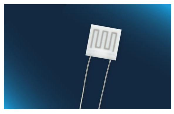
Micro heater for high temperatures up to 850°C based on Zirconia
