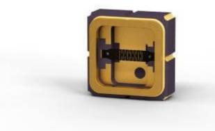
Thermal infrared emitter in standard (3x3) mm<sup>2</sup> SMD package
