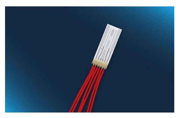
Optimal for applications with a conductivity measuring range from 100  $\mu$ S/cm to 200 mS/cm (typical cell constant of 0.86 cm <sup>-1</sup>) with integrated Pt1000 temperature sensor
